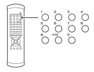
Use the +10 button and 0 through 9 buttons in exactly the same way as when selecting tracks.
